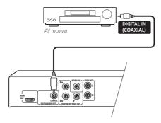
Use a coaxial cable (similar to the supplied video cable) to connect the **COAXIAL DIGITAL AUDIO OUT** jack to a coaxial input on your AV receiver.
